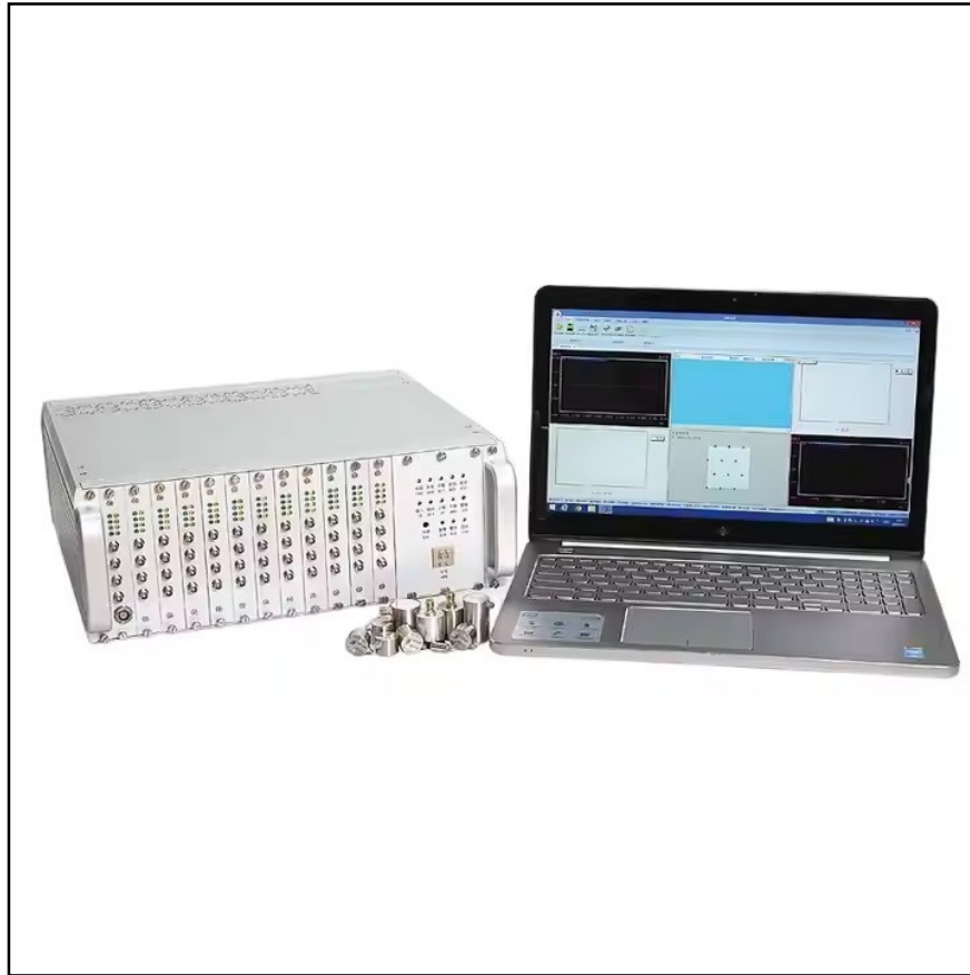
Acoustic Emission Testing (AE) Equipment
