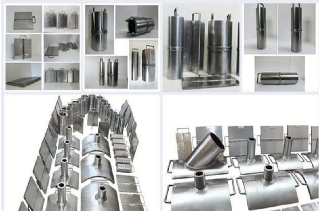
Flawed Specimen Test Components
