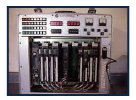
**Allen Bradley WS5610 PLC** Simulator PLC5
