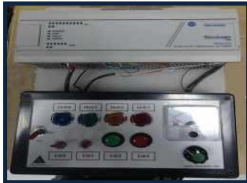
Allen Bradley Micrologix 1000 Simulator (Analog)
