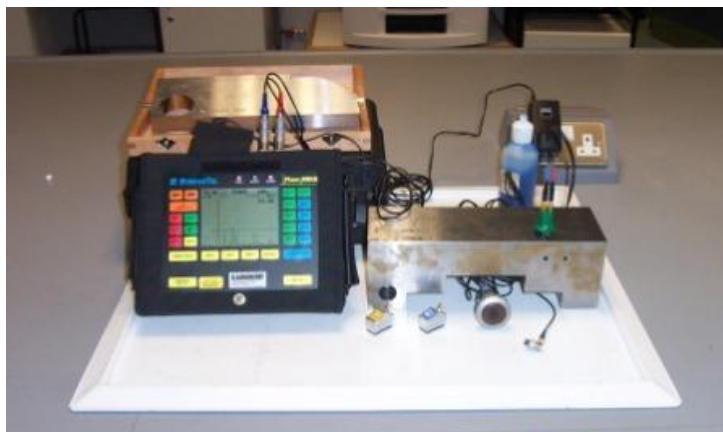
Ultrasonic Testing (UT) Equipment
