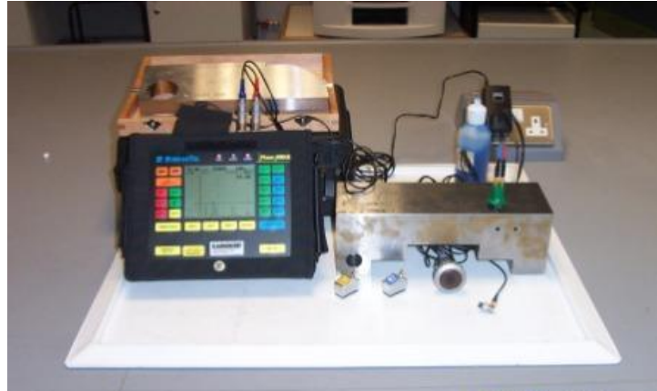
Ultrasonic Testing (UT) Equipment
