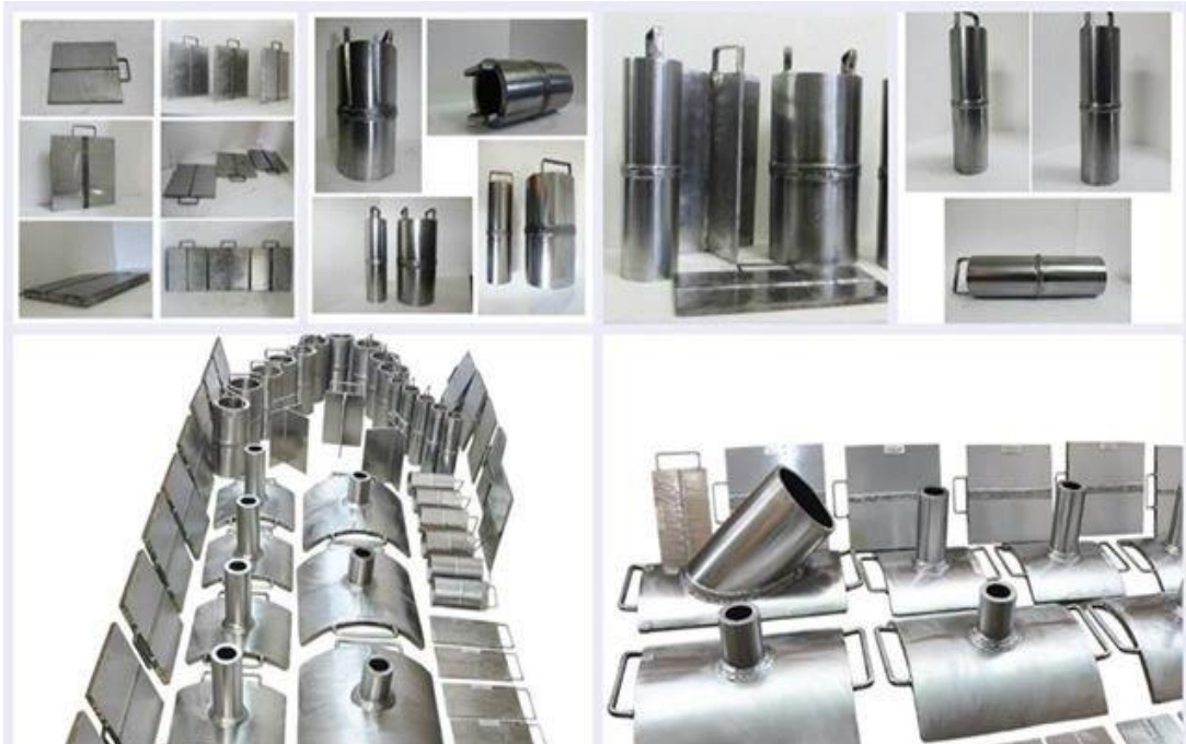
Flawed Specimen Test Components
