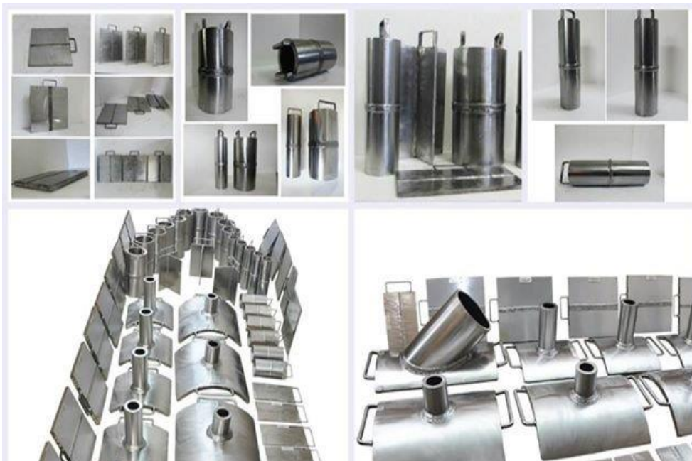
Flawed Specimen Test Components
