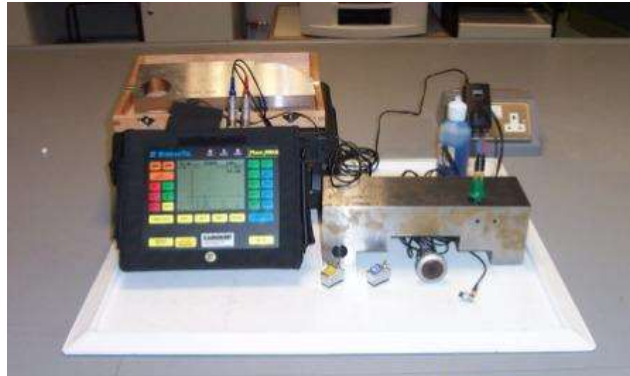
Ultrasonic Testing (UT) Equipment
