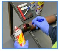
The course covers group discussions around practical problems and provides field expertise on how to resolve them. Participants will be able to employ the liquid penetrant processing including the preparation of parts, adequate lighting, application of penetrant to parts, removal of surface penetrant, developer application and drying as well as inspection, evaluation and post cleaning.
