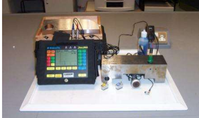
Ultrasonic Testing (UT) Equipment
