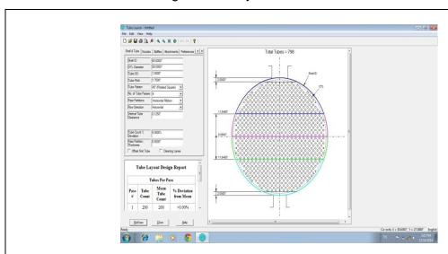
**Heat Exchanger Tube Layout Simulator**
