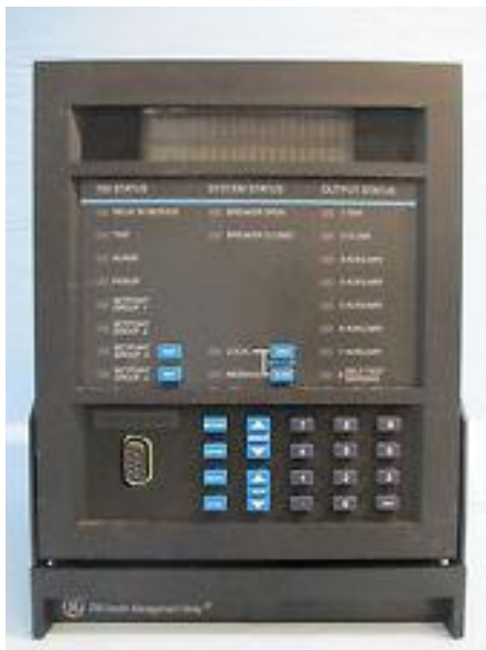
GE Multilin Relay 469 Simulator
