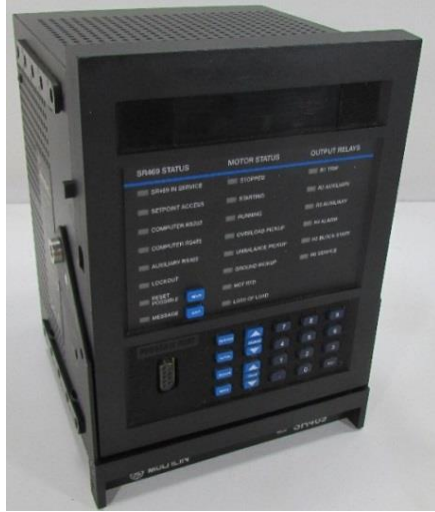
GE Multilin Relay 469 Simulator
