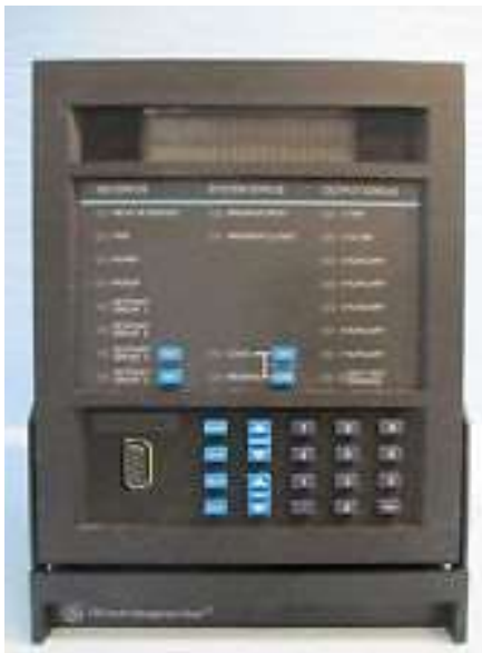
GE Multilin Relay 469 Simulator
