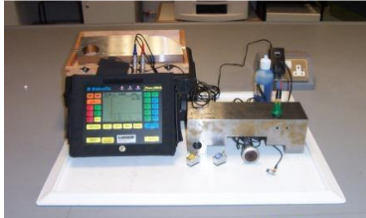
Ultrasonic Testing (UT) Equipment
