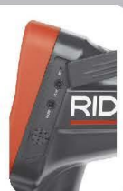
Speaker, Mic, Head Set Jack, AC Power Input
