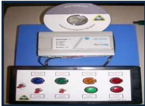
Allen Bradley Micrologix 1000 Simulator (Digital)
