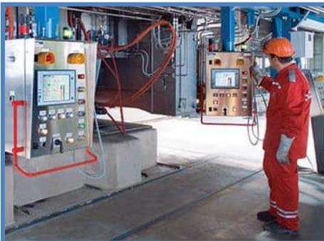
SCADA encompasses the collecting of the information via a RTU (Remote Terminal Unit), transferring it back to the central site, carrying out any necessary analysis and control and then displaying that information on a number of operator screens or displays. The required control actions are then conveyed back to the process.
