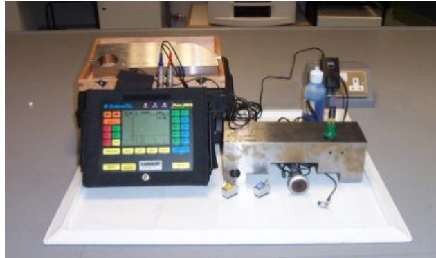
Ultrasonic Testing (UT) Equipment
