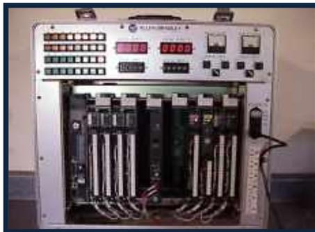
**Allen Bradley WS5610 PLC Simulator PLC5**
