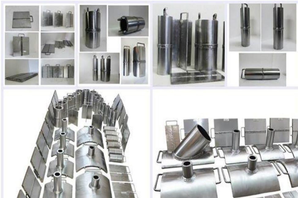
Flawed Specimen Test Components
