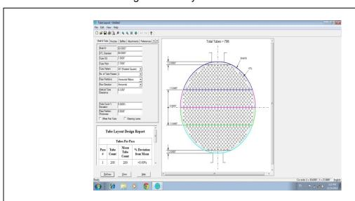
**Heat Exchanger Tube Layout Simulator**
