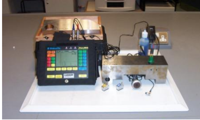
Ultrasonic Testing (UT) Equipment
