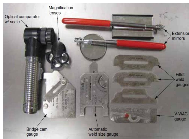
Visual Testing (VT) Equipment
