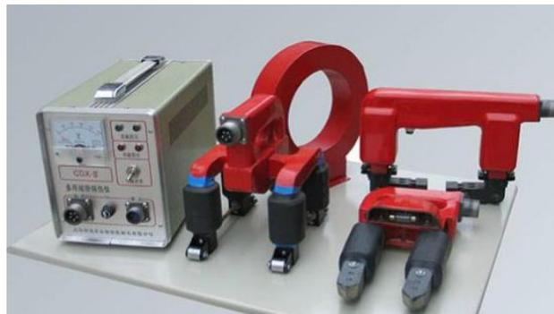
**Magnetic Particle Testing (MT) Equipment**
