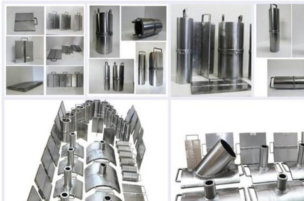
**Flawed Specimen Test Components**
