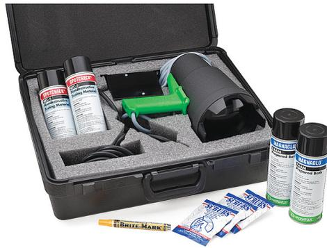
**Liquid Penetrant Testing (PT) Equipment**
