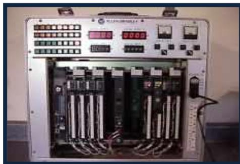
**Allen Bradley WS5610 PLC Simulator PLC5**
